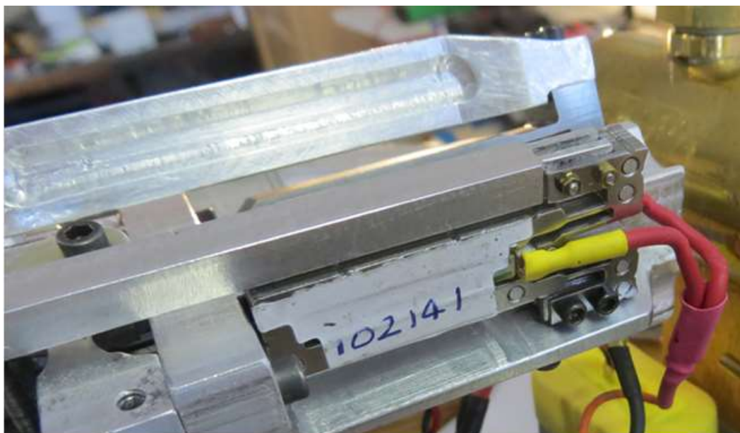
Two 3mm ViVa Actuators with a common actuator arm control the Intake Valve
